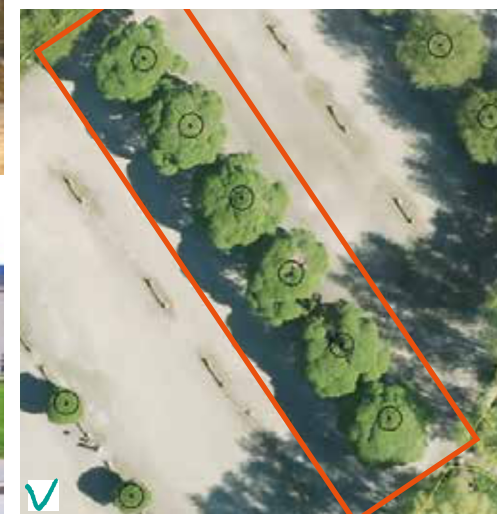
The fence is placed beyond the trees' drip line. No materials may be stored inside the fence. No traffic or machinery may move inside the fence.
